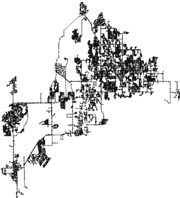
Fig. 2 Placement of Network2 in BWSN (12,523 nodes, 2 sources, 2 tanks, 14,822 pipes, 4 pumps, 5 valves) [8]
