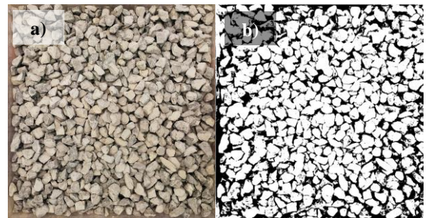
Fig. 3. Plan view of the ballast-filled methacrylate tank, from Test 1. (a): the raw picture taken with a photocamera suspended in the air above the center of the formwork. (b): the binary image obtained from the processing of the raw picture.
