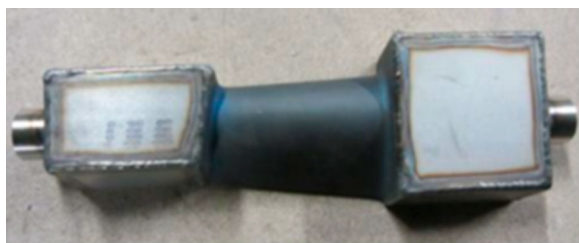
7 The boxes fitted the blade root and shroud to the blades' modified cooling air supply and partial exit, respectively. The blade root (cooling air inlet) is to the right. The blade shroud (main cooling air exit) is to the left
