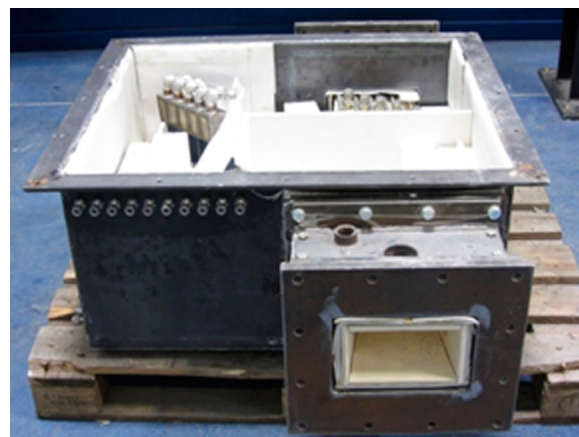
8 Photograph of cascade midway through its construction. The cascade inlet is at the front right, and outlet at the back. In the top left, the third and final stage of cascade blades can be seen
