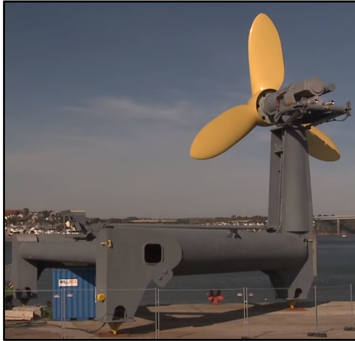
Figure 9 - Prototype Deltastream tidal turbine 32
