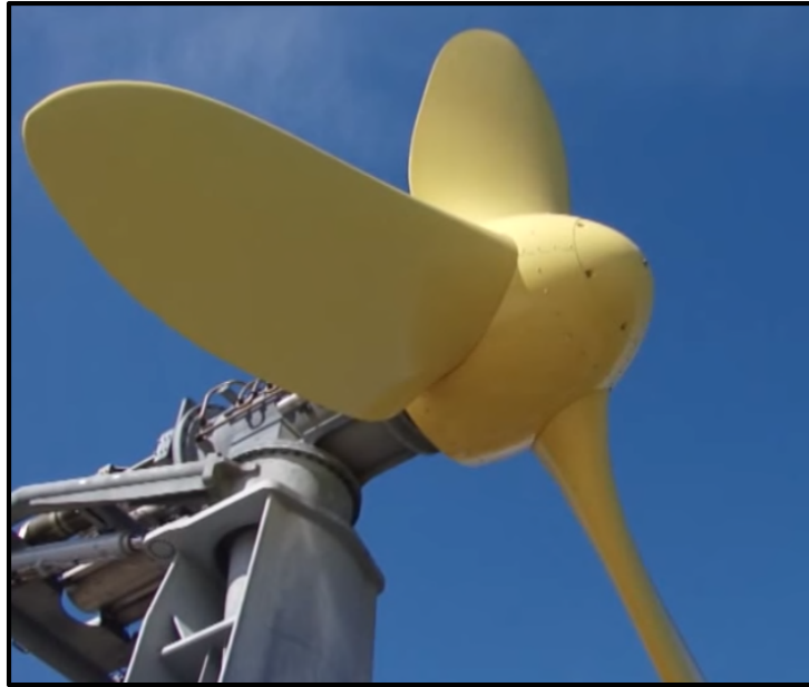
Figure 10 - Prototype Deltastream turbine rotor 32
