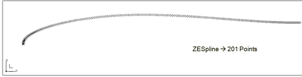
Fig. 6.8. Example of C3 profile exported as a set of points from Matlab ® and imported into CATIA ® v5.
