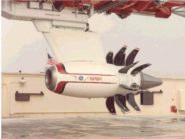
Fig. 3.4. The UDF engine mounted on its ground test rig (source: http://www.cjdbynet , June 2008).
