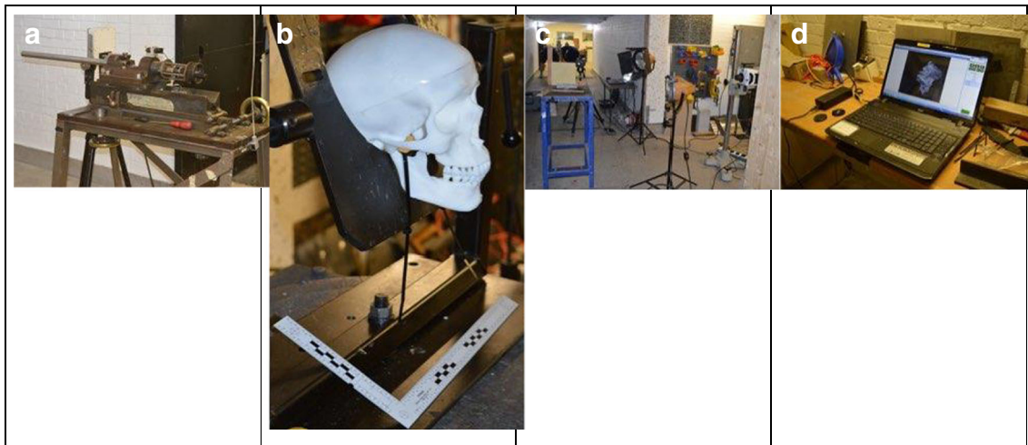
Fig. 2 Experimental setup. a Enfield proof mount. b Skull-brain model. c Camera and lighting setup. d Image capture on laptop PC
