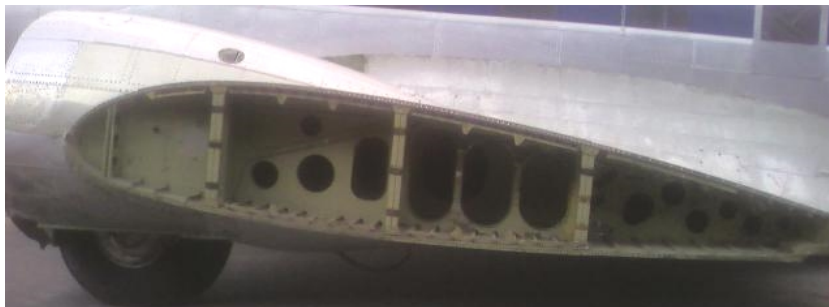
FIGURE 4.5: A photograph showing a cross-section of an aircraft wing.
