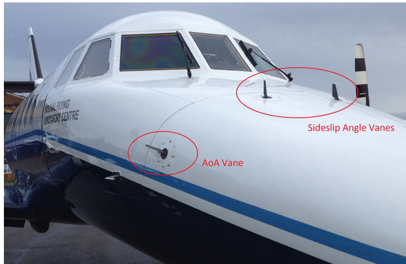
Figure 1: Angle of attack (AoA) vane and sideslip angle vane placement on the BAe Jetstream 3102
