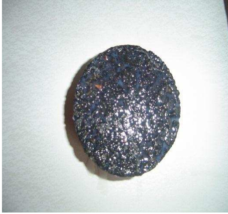
Fig 3. N-doped TiO 2 asphalt road material sample
