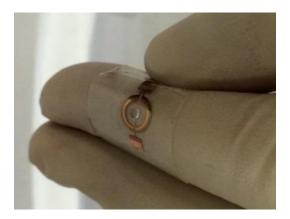
**Figure 2.5** A picture of a device prototype. The center part of the membrane was clear and transparent. The outer copper ring was used to connect the graphene to the external contact pads.
