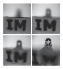
Figure 1.8 Focusing ability of an EWOD lens at different voltages [41].
