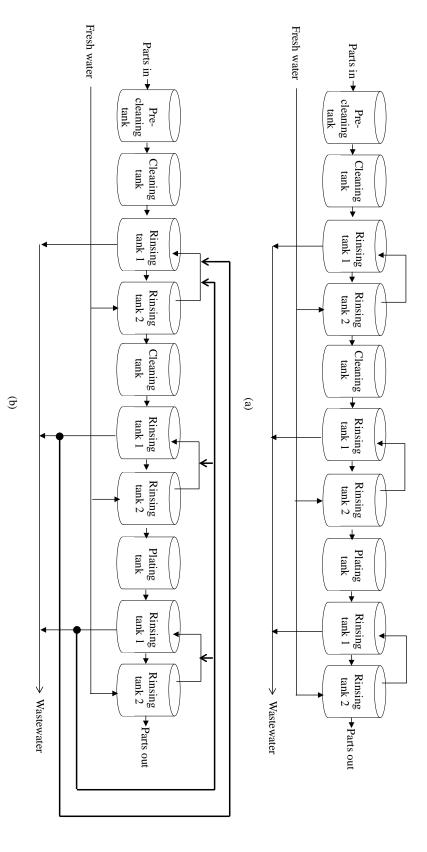
Figure 5.5. Water use and reuse in a plating line: (a) the original process flow sheet, and (b) the new process flow sheet with an embedded optimal water use and reuse network design technology.
