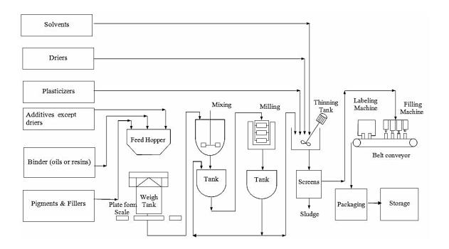
Figure 2.4. Paint manufacturing process (Wikimedia Commons, 2012).
