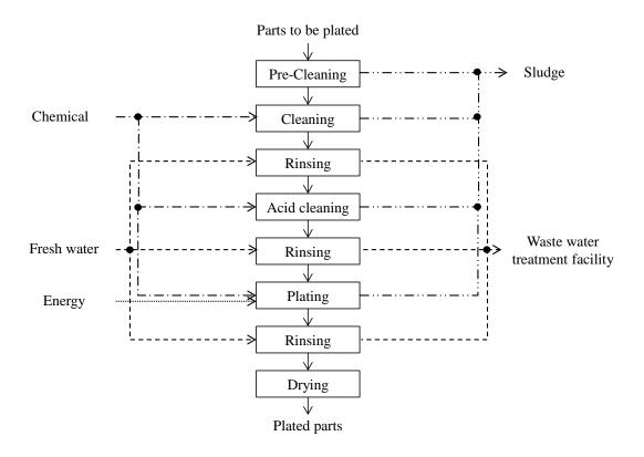
Figure 5.3. Typical electroplating process.
