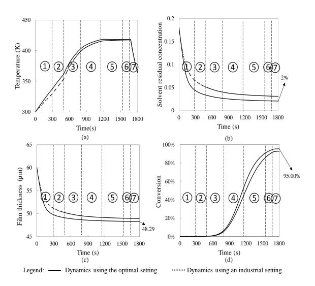
Figure 4.2. Coating performance under new oven operational setting: (a) coating temperature profile; (b) concentration of solvent residual in nanoclearcoat; (c) thickness of nanoclearcoat; (d) conversion rate of cross-linking reaction in nanoclearcoat.
