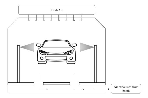
Figure 2.5. Schematic of paint spray booth.
