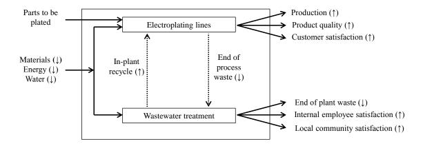
Figure 5.1. Sketch of an electroplating plant with sustainability concerns.
