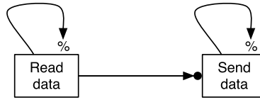
Fig. 5. Simple DCR graph of a read-send process.
