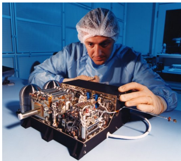
Fig 2 shows an Open University scientist working on 'Ptolemy', the advanced and miniature chemical and isotopic analysis laboratory currently flying on board the ESA Rosetta lander Philae. Credit The Open University / CCLRC Rutherford Appleton Laboratory.
