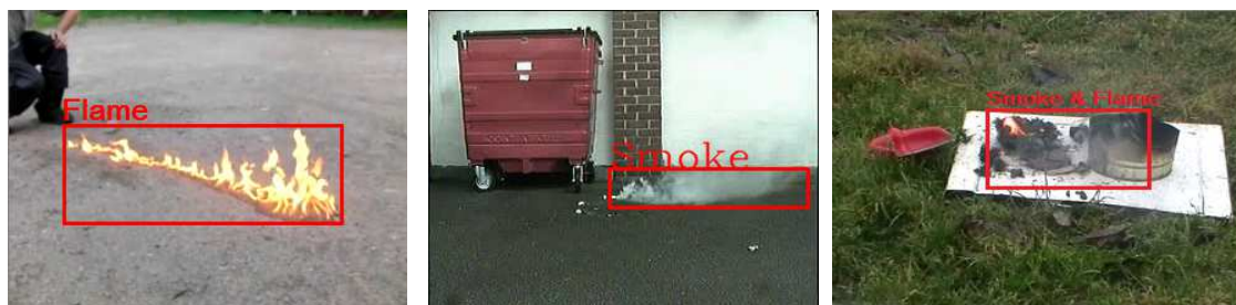
Fig.1. Examples of smoke and flame detection with a hybrid algorithm
