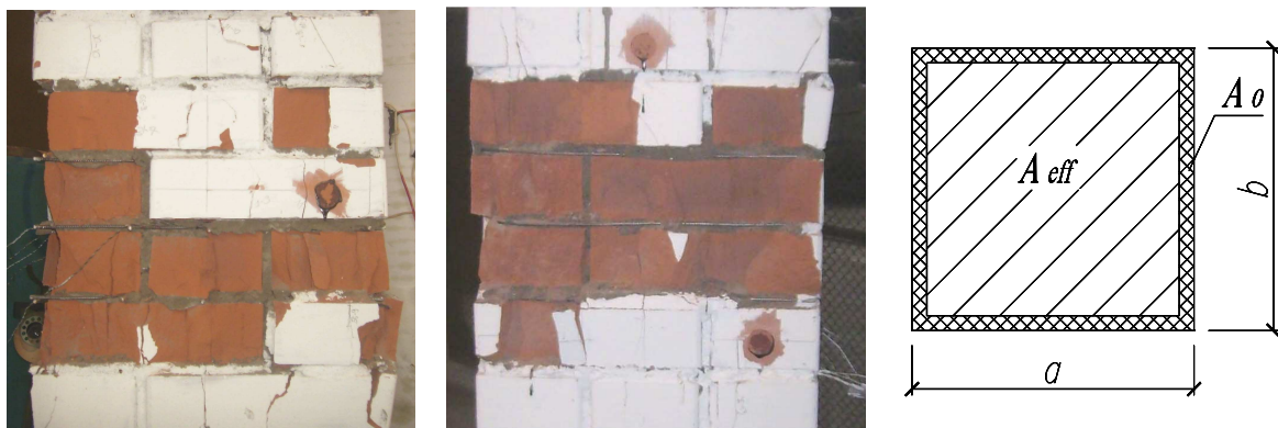
Fig. 1. Character of destruction reinforced samples, division section on A_{eff} and A_0
