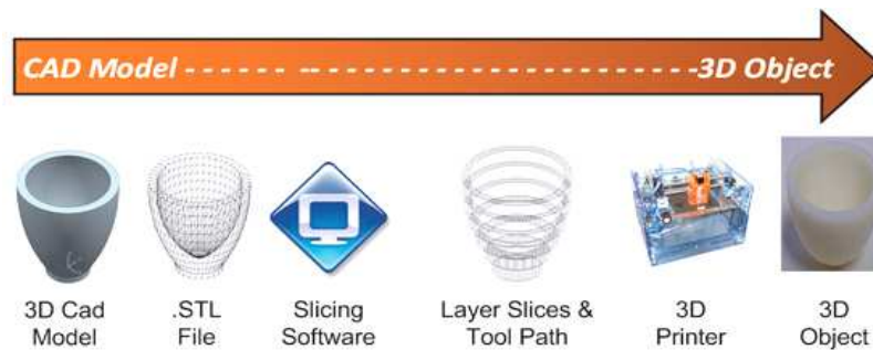
Fig. 3. Stages of manufacture: from modeling to fabrication of a physical body
