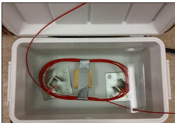
Figure 2: Experimental layout of each temperature calibration; a TidBit temperature logger placed on the wooden block suspended in the center of the coil provided a representative temperature measurement at the same depth as the cable. The aquarium pump was placed beneath the wooden block, and the heating unit was attached horizontally near the water surface, parallel to the long side of the cable coil.
