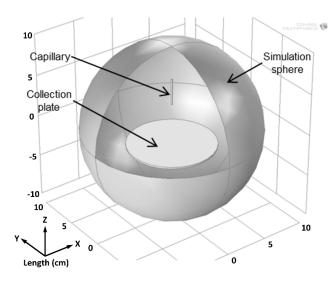
Figure 5: *COMSOL* simulation sphere containing the collection plate and capillary. The simulation assumes that the electric field is not influenced by the surroundings. Reprinted with permission from Beisel, Joshua D., et al. "Analytical parametric model used to study the influence of electrostatic force on surface coverage during electrospinning of polymer fibers." *Journal of Vacuum Science & Technology B* 32.6 (2014): 06FI03. Copyright 2014, American Vacuum Society.
