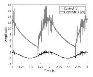
Figure 12: Sinusoidal 1 Hz control voltage and output voltage that is applied to the electrodes. The changing electric field causes the ES fiber to preferentially deposit to one electrode then the other as the voltage changes. Reprinted with permission from Beisel, Joshua D., et al. "Lithography via electrospun fibers with quantitative morphology analysis." *Journal of Vacuum Science & Technology B* 34.6 (2016): 06KG02. Copyright 2016, American Vacuum Society.
