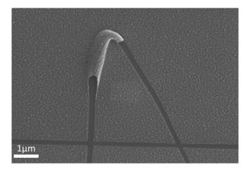
Figure 18: Incomplete lift-off of the aluminum thin film. Defects such as this are caused by a conformal coating of aluminum on the electrospun fiber. Adjusting the process parameters these defects were reduced.
