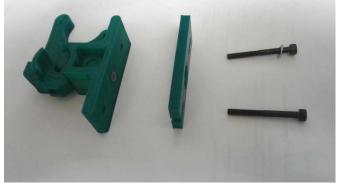
Figure 36: LulzBot(R) Flexystruder print head. This print head offers continual filament support which is required when printing with NinjaFlex®.
