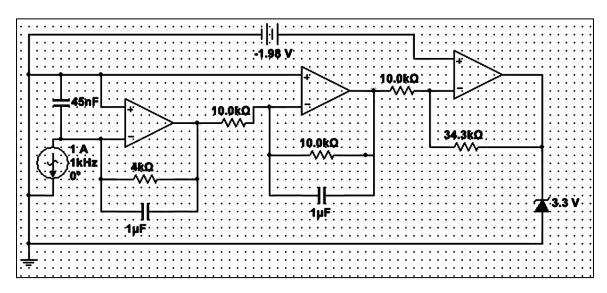
Figure 27: Circuit schematic of LaD circuitry. The node output from op-amp that is connected to the Zener is also connected to the microcontroller. An alternating current source was used in place of a photodiode to simulate the response characteristics and analyze the circuit stability.
