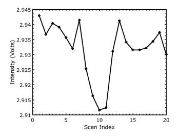
Figure 31: Reduction in laser intensity as the LaD system scans through the candle flame. The reduction is caused by the interaction between the laser and the soot particles such as reflection, refraction, and absorption which are grouped together as a measurement of laser extinction.
