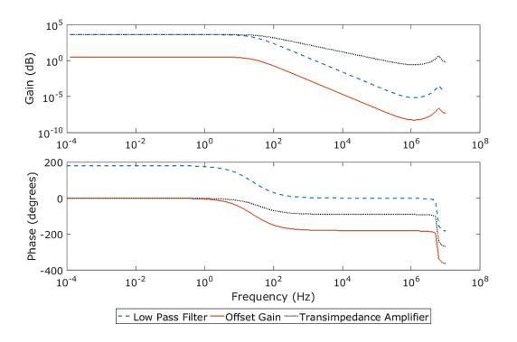
Figure 35: Frequency response of the LaD circuitry. The gain margin and phase margin of the response confirm circuit stability.
