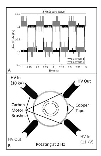
Figure 13: Square-wave signals (A) generated from the commutator (B). The input voltages are 10 kV and 11 kV which generates two 1 kVpp square-wave signals that are 180° out of phase. Reprinted with permission from Beisel, Joshua D., et al. "Lithography via electrospun fibers with quantitative morphology analysis." *Journal of Vacuum Science & Technology B* 34.6 (2016): 06KG02. Copyright 2016, American Vacuum Society.
