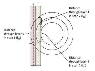
Figure 4: Laser interrogating ES fibers during deposition. The layers that are created for each scan demonstrate the onion-peel deconvolution process.
