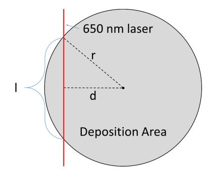
Figure 23: The length that the laser travels through the area of deposition is used in the onion-peeling deconvolution method to calculate the extinction coefficient of an annular region of the fibers that are being deposited. Through calibration curves, the extinction coefficient will be used to determine the diameter of the fibers being deposited.
