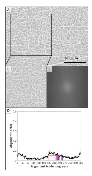
Figure 16: A random fiber sample (A) was deposited onto a single electrode for comparison. FFT analysis was completed on the random deposition follow the procedure used on aligned fibers. A 512-pixel square was cropped from the image (B) followed by 2-D FFT analysis (C). The wide bandwidth and low alignment factor provide baseline comparison values (D). Reprinted with permission from Beisel, Joshua D., et al.
