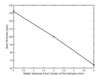
Figure 32: Soot-volume fraction through a tea candle as calculated from LaD measurements. The size of the candle flame in combination with the spot size of the laser allowed for the soot concentration to be calculated in three annular regions of the candle.
