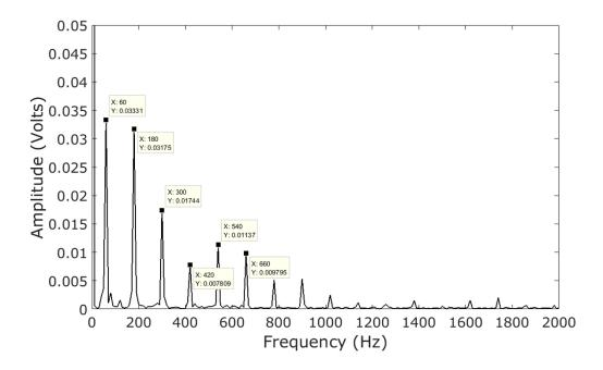
Figure 25: Frequency analysis of original fabricated power supply. Noise levels ranging from 5 mV to 33 mV contributed to the low signal to noise ratio of the laser extinction measurements.
