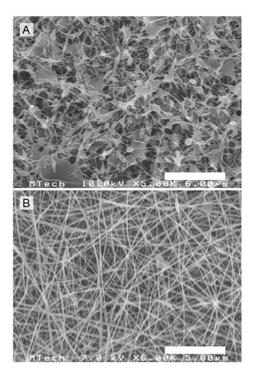
Figure 7: SEM of ES PVA fibers. The beaded fibers (A) were the result of 4 wt% PVA, whereas the uniform fibers (B) were the result of 6 wt% PVA. Reprinted with permission from Beisel, Joshua D., et al. "Analytical parametric model used to study the influence of electrostatic force on surface coverage during electrospinning of polymer fibers." *Journal of Vacuum Science & Technology B* 32.6 (2014): 06FI03. Copyright 2014, American Vacuum Society.
