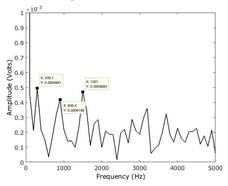
Figure 26: Frequency analysis of HIPRO power supply. The signal conditioning provided by the HIPRO power supply decreased the amount of electrical noise on the system which increased the signal to noise ratio of the extinction measurements.
