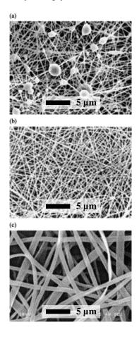
Figure 21: Various fiber morphologies of ES PVA at various molecular weights. Each solution is at 25 wt%. The 9 000-10 000 g/mol MW resulted in beaded fibers (a); 13 000-23 000 g/mol MW resulted in fiber with a circular morphology (b); and 31 000-50 000 g/mol MW PVA resulted in flat fibers (c). Reprinted from Materials Letters, Vol 58, A. Koski, K. Yim, S. Shivkumar, Effect of molecular weight on fibrous PVA produced by electrospinning, 493-497, Copyright 2004, with permission from Elsevier.
