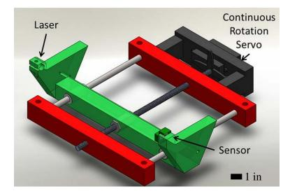
Figure 3: Original laser diagnostics tool setup. This setup utilized a continuous rotation servo motor and an additive manufactured linear stage to move the laser and sensor simultaneously.
