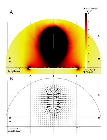
Figure 8: Heat map (A) and vector field (B) of the electric field generated from the *COMSOL* model with a separation distance of 4.0 cm and an applied voltage of 15 kV. Reprinted with permission from Beisel, Joshua D., et al. "Analytical parametric model used to study the influence of electrostatic force on surface coverage during electrospinning of polymer fibers." *Journal of Vacuum Science & Technology B* 32.6 (2014): 06FI03. Copyright 2014, American Vacuum Society.
