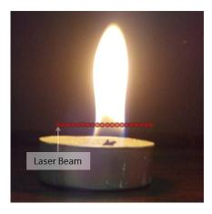
Figure 24: Synthetic image of the LaD system scanning through a candle flame to calculate the soot-volume fraction of the concentric layers of the candle. The amount of transmitted light from the laser is measured through the flame is measured as a voltage and compared to the initial intensity of the laser to calculate the amount of extinction that has occurred due to the soot particles that were generated.
