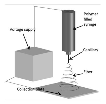
Figure 1: Basic electrospinning setup where a polymer delivery system is connected to a capillary. A high voltage power supply applies a DC voltage potential between the capillary and the collection plate.
