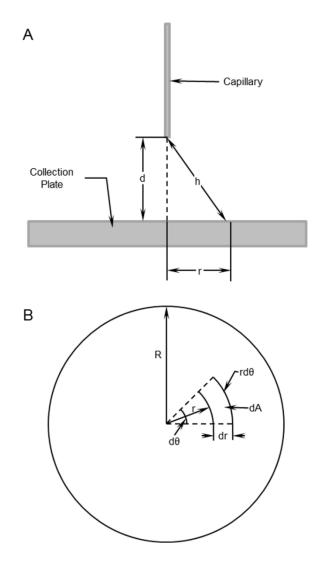
Figure 6: ES setup from the side view (A) defining measurements inside the electrospinner. A top view of the collection plate (B) defines the differential area parameters where the collection plate is centered on the capillary. Reprinted with permission from Beisel, Joshua D., et al. "Analytical parametric model used to study the influence of electrostatic force on surface coverage during electrospinning of polymer
