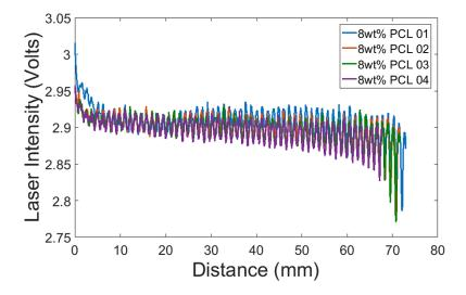
Figure 29: Sinusoidal noise induced from the misalignment between the stepper motor and the linear stage drive shaft. The period of the induced signal is equal to one revolution of the stepper motor.
