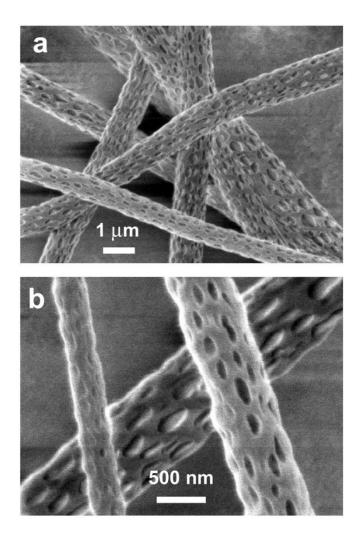
Figure 20: Micrograph of porous fibers fabricated from a PLLA dichloromethane solution (a) with magnification of the porous structures (b). Reprinted with permission from Bognitzki, Michael, et al. "Nanostructured fibers via electrospinning." Advanced Materials 13.1 (2001): 70-72. Copyright 2001, Advanced Materials.
