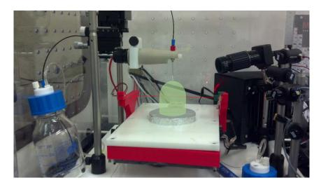
Figure 28: Initial construction of the LaD system installed in a SprayBase® electrospinner with added graphics to depict the interaction between the laser and the fibers during deposition. The laser and sensor simultaneously move to measure the amount of laser extinction due to the fibers being deposited.
