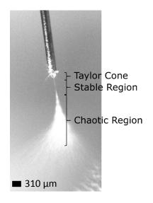
Figure 2: Regions of ES deposition. With near-field ES the collection plate is within the stability region of the fiber; whereas with far-field ES the collection plate is in the unstable/chaotic region of the fiber.
