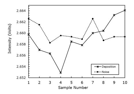
Figure 33: Extinction caused by ES fibers compared to noise floor of the sample. Interactions between the laser and the fibers were visually observed for sample numbers 2-4 with corresponding laser extinction measurements.
