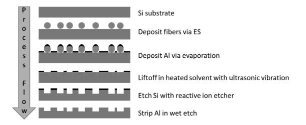
Figure 14: Process to pattern transfer the ES fibers onto a silicon substrate through RIE. Reprinted with permission from Beisel, Joshua D., et al. "Lithography via electrospun fibers with quantitative morphology analysis." *Journal of Vacuum Science & Technology B* 34.6 (2016): 06KG02. Copyright 2016, American Vacuum Society.
