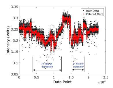
Figure 34: Laser extinction through PEO fibers at a 100 sps data rate. The fiber deposition was scanned twice, the data points designated as "in field of deposition" correspond to points where the interactions between the laser and the fibers were visually confirmed.
