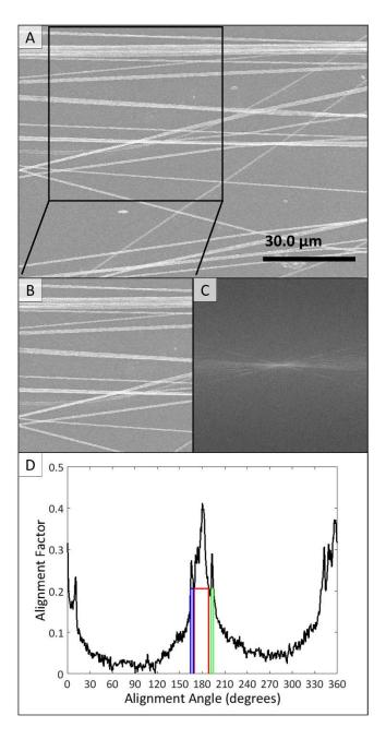
Figure 17: Fiber deposition occurred between right electrodes (A). A section of sparse fibers (B) was analyzed with a 2-D FFT (C). The sparse deposition revealed a combined bandwidth of 26.28° with a peak alignment factor of 0.4114 (D). Reprinted with permission from Beisel, Joshua D., et al. "Lithography via electrospun fibers with quantitative morphology analysis." *Journal of Vacuum Science & Technology B* 34.6 (2016): 06KG02. Copyright 2016, American Vacuum Society.
