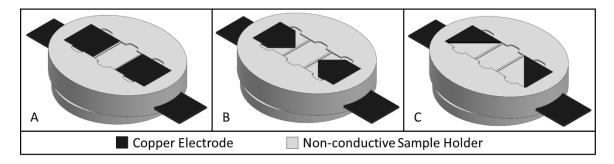
Figure 11: Independently controlled copper electrodes with square (A), obtuse (B), and right (C) geometries were placed on glass with room between the electrode pairs to place a removable collection plate. Reprinted with permission from Beisel, Joshua D., et al. "Lithography via electrospun fibers with quantitative morphology analysis." *Journal of Vacuum Science & Technology B* 34.6 (2016): 06KG02. Copyright 2016, American Vacuum Society.
