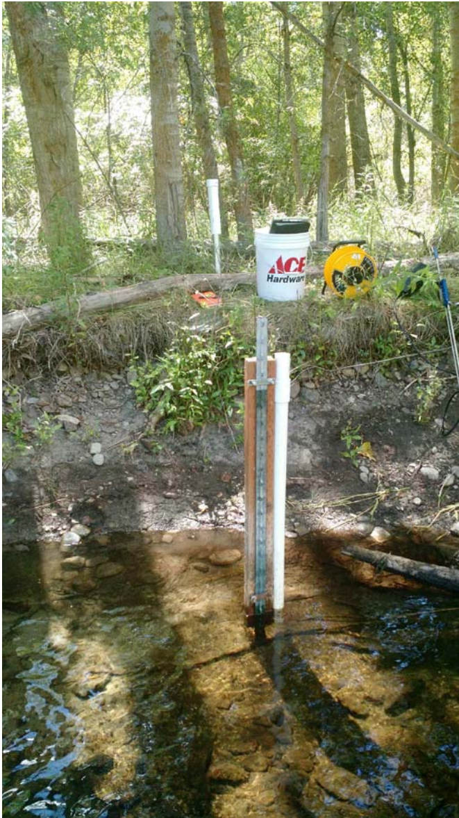
Figure 10: Instrumentation setup with staff gage in the stream and piezometer on the bank.
