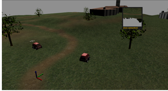
Figure 2.6. Screenshot of outdoor simulation in MORSE with two mobile and one aerial robot.
