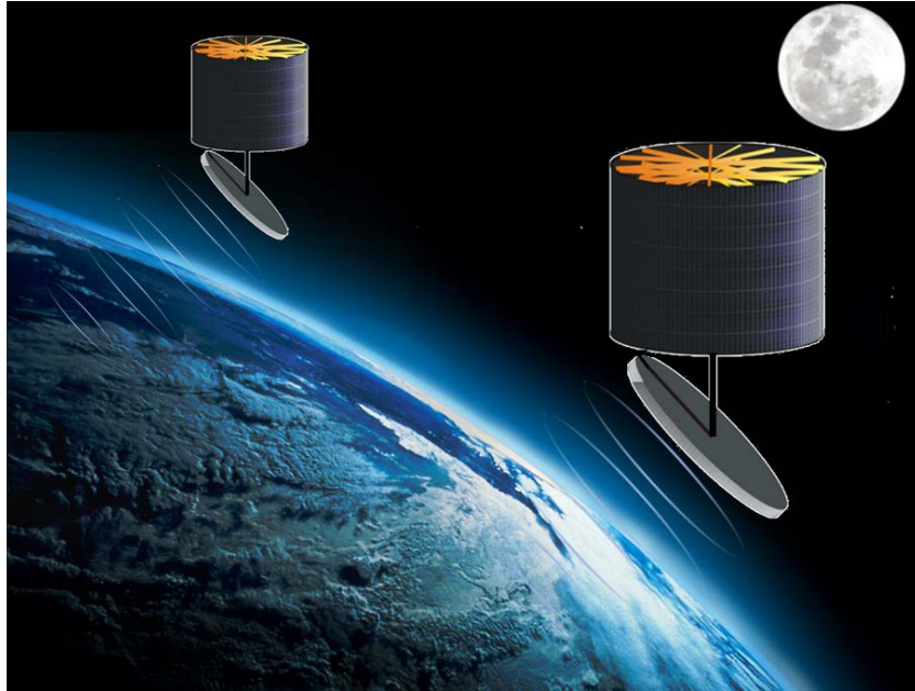
Figure 1. Solar Power Satellites (SPS) collecting sunlight in orbit and delivering Wireless Power Transfer (WPT) to terrestrial receiving antennae. This system is called Space Solar Power (SSP).
