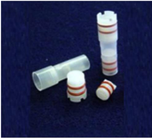
Figure 13. PULSE tube FT500. The ram transmits pressure to the sample and the screw cap seals the tube. The sample lies on top of the lysis disk filled with perforations that allow sample to be pushed into the collection chamber. Adapted for Pressure BioSciences, Inc. website.
