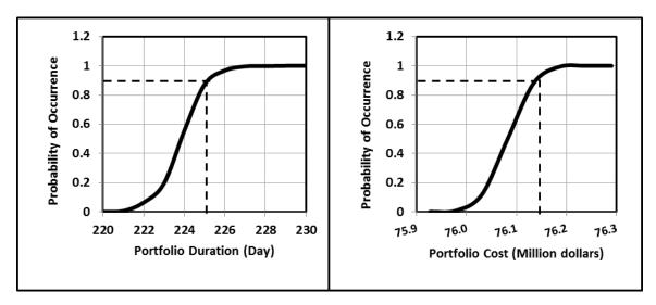
Figure 4.5. Extracting portfolio duration and cost from stochastic simulation outputs (distributions) based on pre-defined confidence levels
