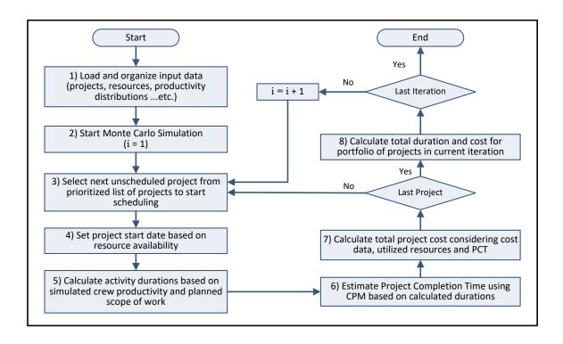
Figure 3.2. Flowchart for the Monte Carlo simulation procedure
