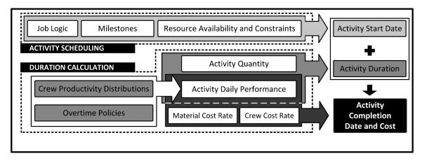
Figure 4.3. Activity level analysis from the simulation module
