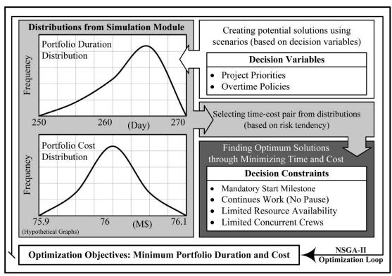
Figure 5.2. Multi-Objective optimization module
