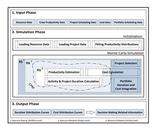
Figure 3.1. Productivity Simulation Model (PSM)
