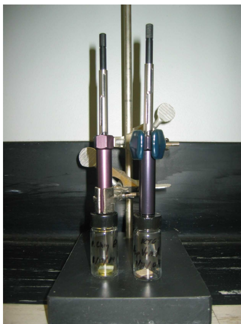
Figure 2. Photograph of initial Solid Phase Microextraction apparatus.
