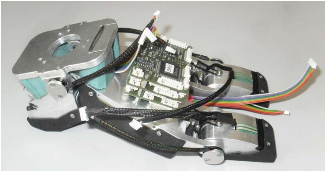
(c) Photograph of the designed and integrated foot structure including its PCB stack. The force/torque sensor, used as the mechanical interface to the ankle joint, is not displayed.
