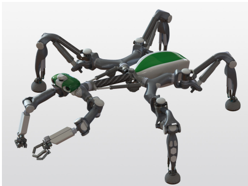
(a) The robot Mantis with its front limbs, which can either be used for manipulation or locomotion tasks. Source: DFKI GmbH RIC.
