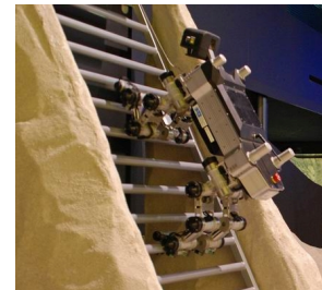
(c) The robot Aramies features actuated claws. Source: DFKI GmbH RIC.
