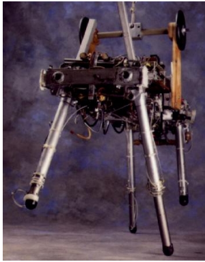
(a) Four-legged walking machine “Quadruped” from MIT. Source: [MIT].
