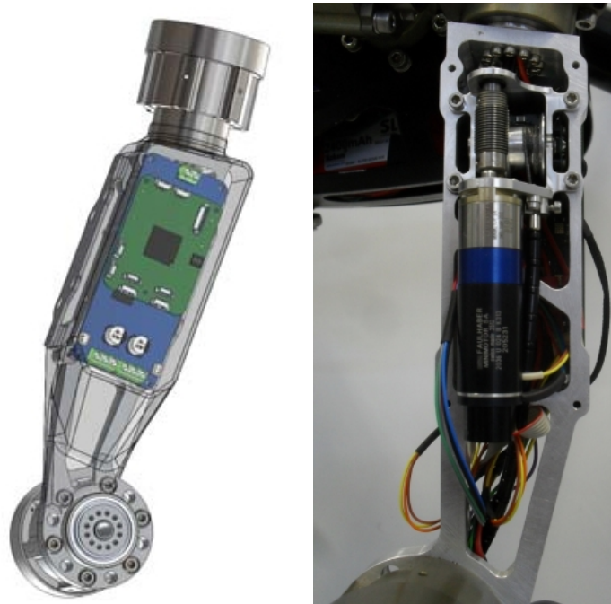
(a) Front view: thigh with electronic stack (CAD rendering). (b) Rear view: photograph of the thigh with installed motor for toe actuation.
