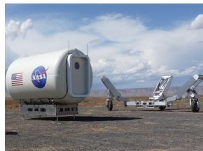
(b) One Tri-ATHLETE unit before docking a cargo-unit. Adapted from: [HMFMQ10].
