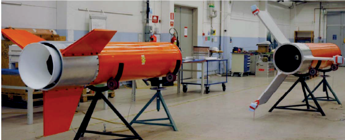
Figure 5.2: VSB 30 motors in integration hall at Esrange [Sta12]
