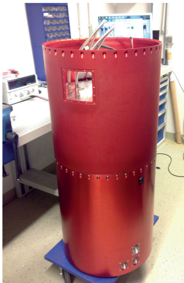
(a) Test setup of upper and lower MAIUS hull segments
