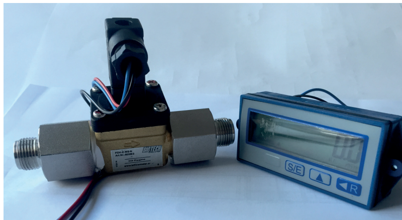
Figure 12.3: Modified flow meter (left) and counter (right) for measurement of the flow rate in the MAIUS cooling circuits.
