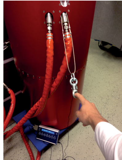
(a) Separation force for six separation tests with the water umbilical connector (b) Test setup for water umbilical
