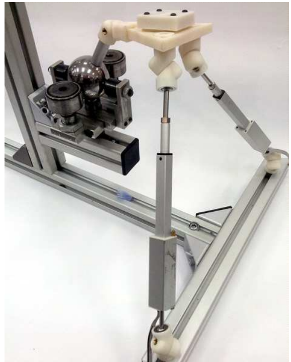
Fig. 1. A simple implementation of the studied non-holonomic parallel orienting robot (see [6] for details).
