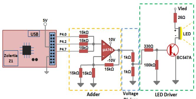
Fig. 5. Transmitter circuit diagram.
