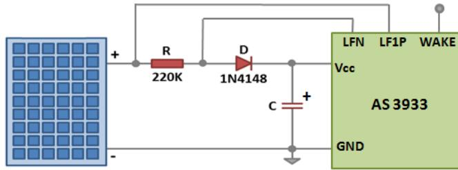
Fig. 2. Circuit diagram of the wake-up receiver.
