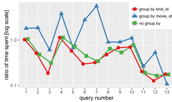
Figure 3.16: Performance gain with eager aggregation by complete enumeration for queries without selectivity
