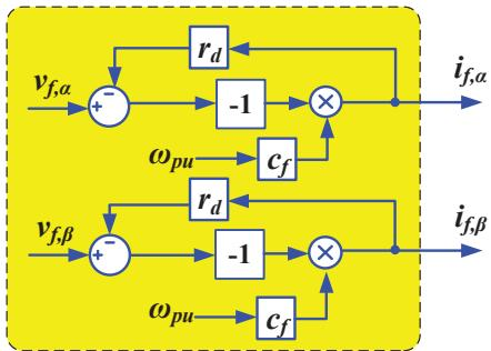
Fig. 3. Estimation of capacitor current for Method 2.
