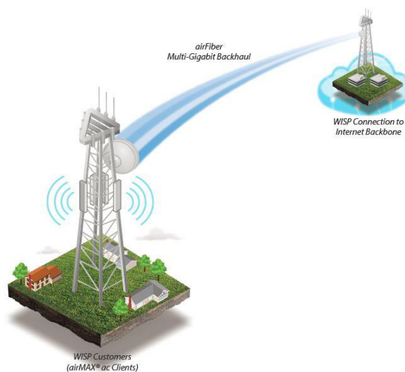
Figure 17 - Ubiquiti Airfiber link
