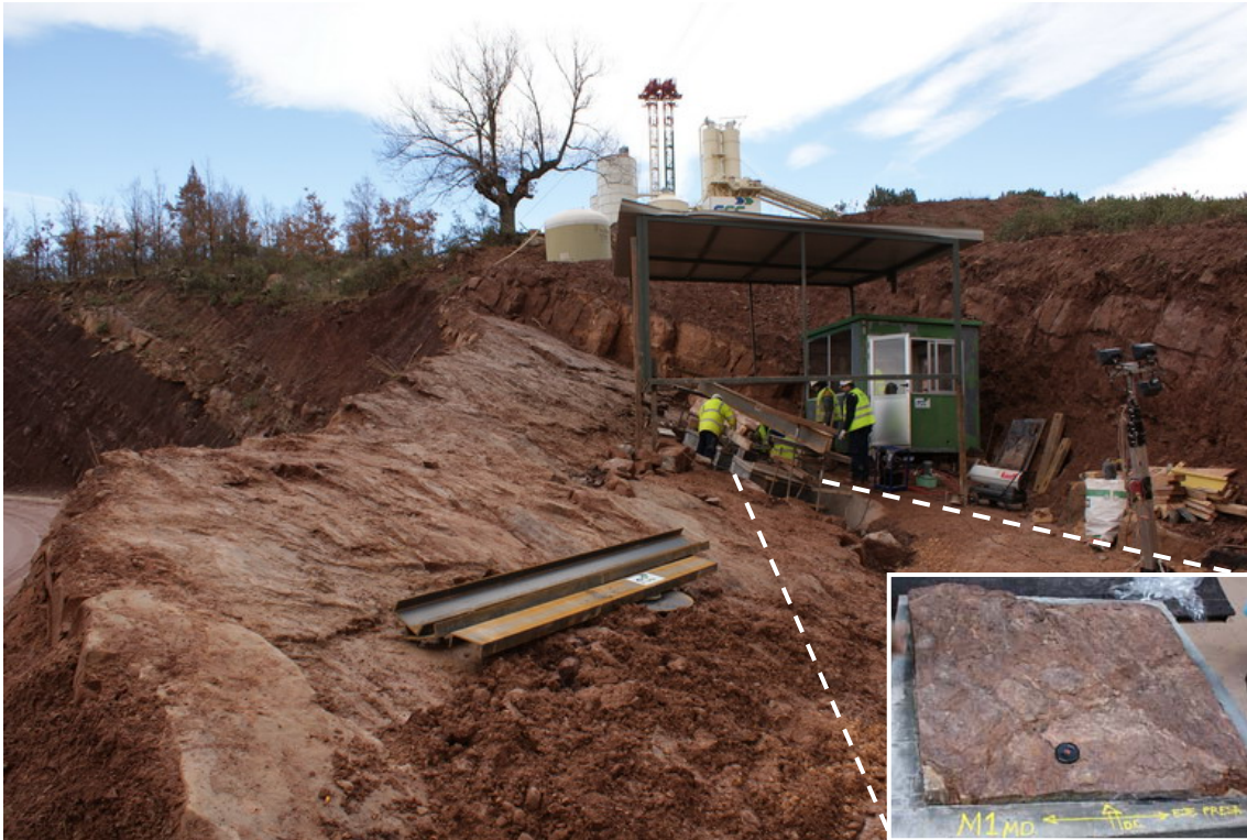
Figure 20: Castrovido Weald form. Exposed sandstone-claystone sedimentation surface. Zoom-in of contact after insitu shearing test.
