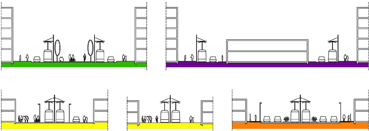
Item 11: Urban territory of Zaragoza and modes of incorporation of the tram in the street profile (own elaboration)
