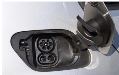
Figura 7.2. Connector CCS del VW e-Golf [20]
