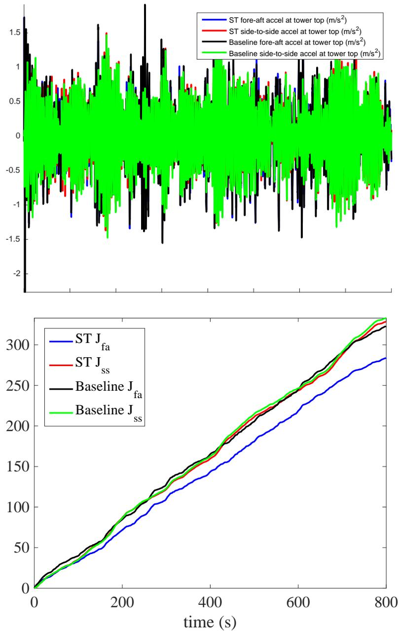
Figure 5: *Fore-aft* and *side-to-side* accelerations (top) and related  $J_{fa}$  and  $J_{ss}$  indices (bottom) at the tower top.
