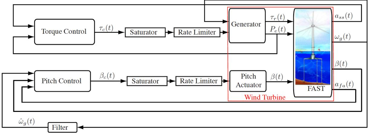
Figure 1: Block diagram of the closed loop system.
