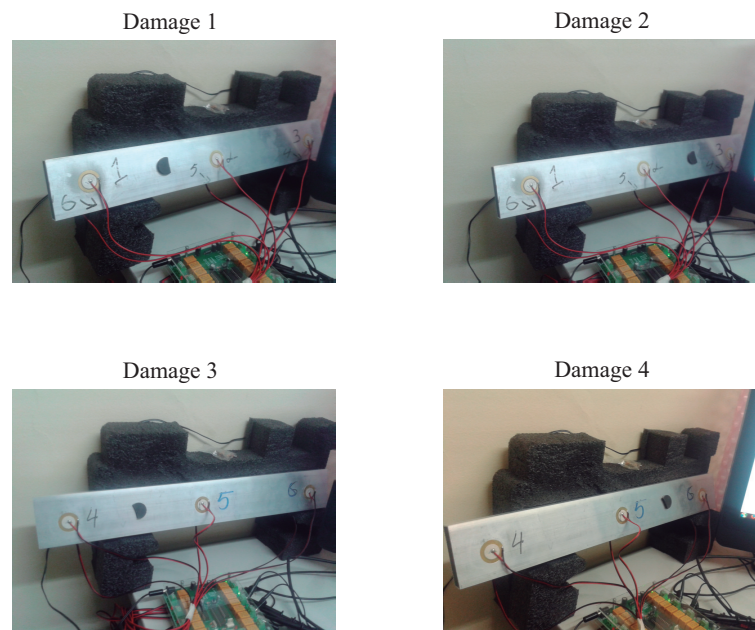
Figure 13. Aluminum rectangular profile instrumented with six piezoelectric sensors and with four different damage.
