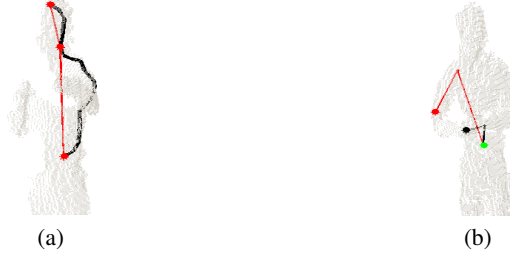
Fig. 3. (a) Approximate geodesic path with mid-band. (b) Benefit of geodesic distance updating.
