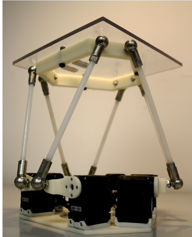
Figure 24: Structure of the parallel robot's manipulators
