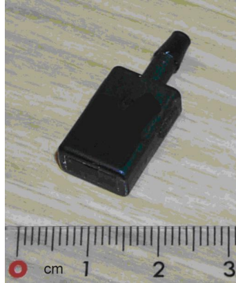
Figure 1.1: Windshield washer fluid dispenser [8]
