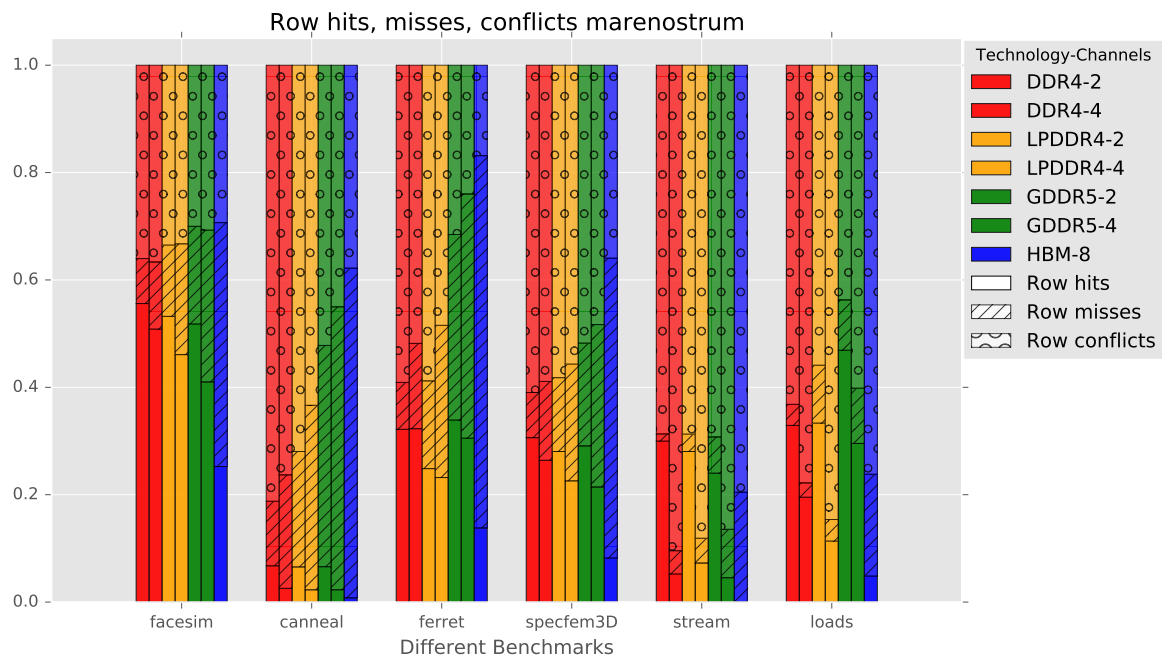
Fig. 6.6 Row hits, misses and conflicts of benchmarks on marenostrom with different memory technologies.
