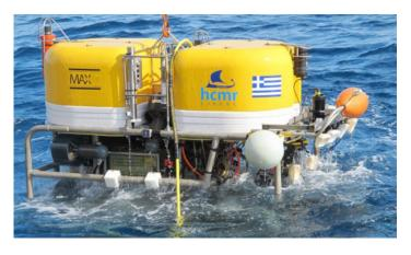
Fig 2. Recovering the ROV Max Rover (HCMR, Greece).
