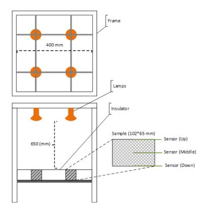
Figure 4. Radiation test setup
