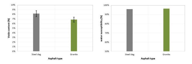
Figure 5. Asphalt mixes voids content
