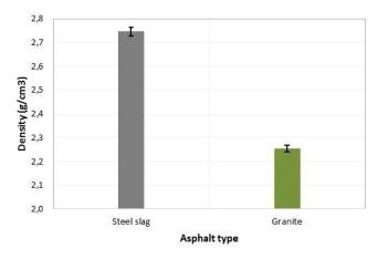
Figure 7. Asphalt mixes density
