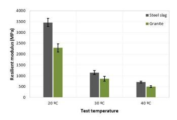
Figure 8. Asphalt mixes resilient modulus at different temperatures
