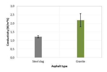
Figure 12. Thermal conductivity (W/m\*K).
