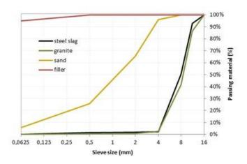
Figure 1. Size distribution of aggregates
