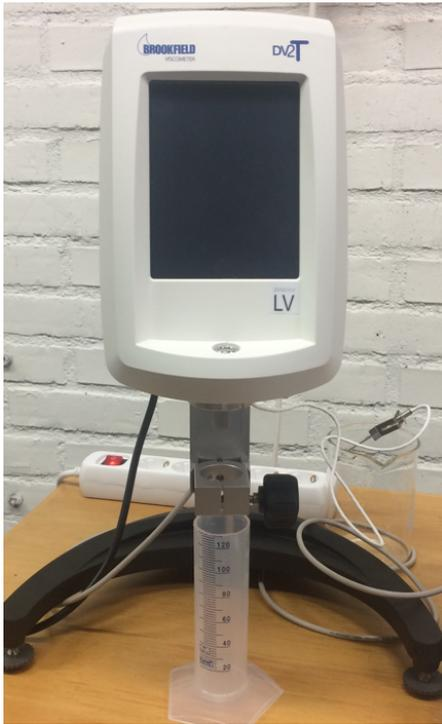
**Figure 3.3:** DV2T Brookfield LV viscometer.
