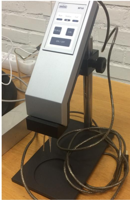
**Figure 3.2:** KRÜSS Bubble pressure tensiometer BP50 used for surface tension measurements.
