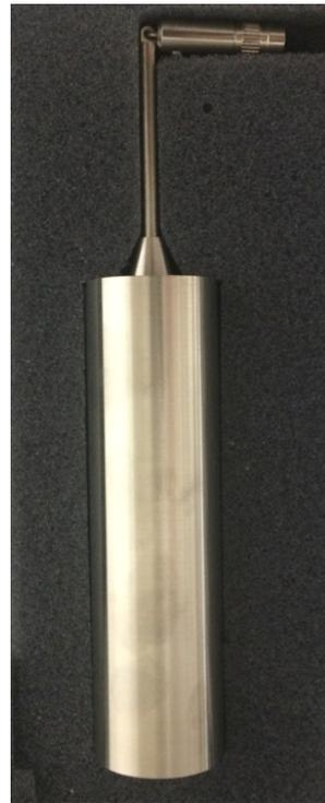
**Figure 3.4:** Ultra low viscosity spindle used in the viscosity test.
