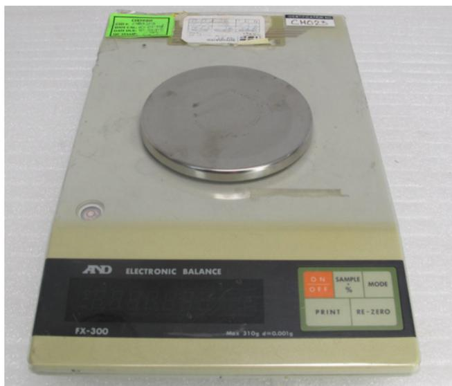
**Figure 3.1:** Electronic balance, FX-300 AND, used for blend preparation and density determination.
