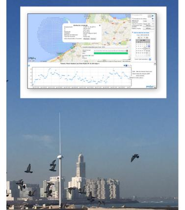
Fig. 6 Compact 2 x 4.5 MHz SeaSonde HF Radar system in Morocco and principal 2D deliverables, currents mapping and waves monitoring. (HF Radar system operated by the Direction de la Météorologie Nationale).
