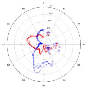
Fig. 3 - Loop patterns in the Espichel HF Radar station. Instituto Hidrografico of Portugal. Legend: red - Loop 1; blue - Loop 2; continuous line - boat pattern; circles - Auto-APM pattern. **Toscana, SICOMAR, Italia.**
