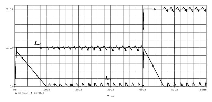
Fig. 7. Detail of the output current  $I_{out}$  and the linear regulator current  $I_{reg}$  at the start transient of the converter in figure 4 with  $V_{in}=10$  V. It can also be observed the response of the circuit to an input voltage step from 10 V to 13 V at  $t=20 \ \mu s$ , and a variation in the load resistance from 5  $\Omega$  a 2.5  $\Omega$  at  $t=40 \ \mu s$ . The switching threshold current  $I_{\gamma}$  is fixed at 5 mA.
