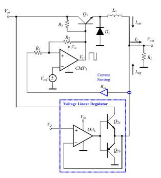
Fig. 4. Basic structure of linear-assisted converter with control strategy 'B'.
