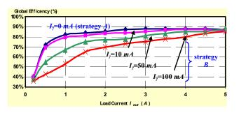
Fig. 8. Experimental efficiency for the control strategy 'A' and the proposed by the authors (strategy 'B') with  $V_{out}=5 V$ . It is shown four different  $I_{\gamma}$  values: 0 mA (strategy A), and 10 mA, 50 mA and 100 mA (all three for strategy 'B').
