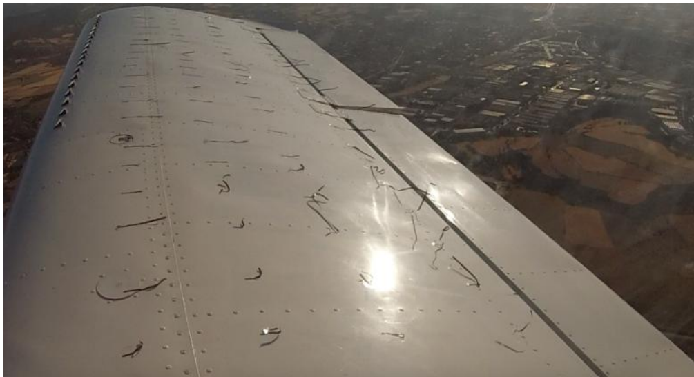
Figure 59: Experimental tests with VG: fully stalled wing
