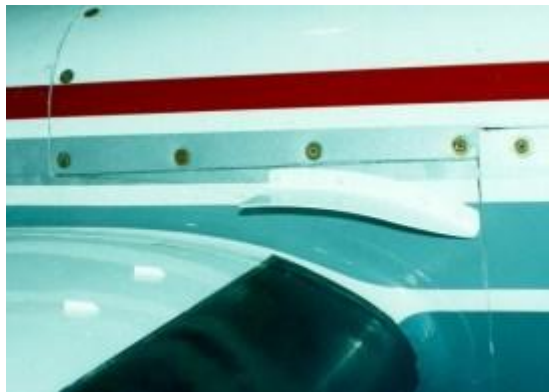
Figure 17: Nacelle vortex generator mounted on a multi-engine airplane. Source [16].
