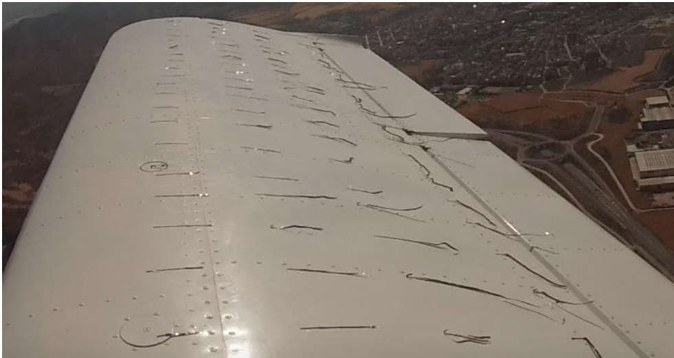
Figure 55: Experimental tests without VG: stall progression
