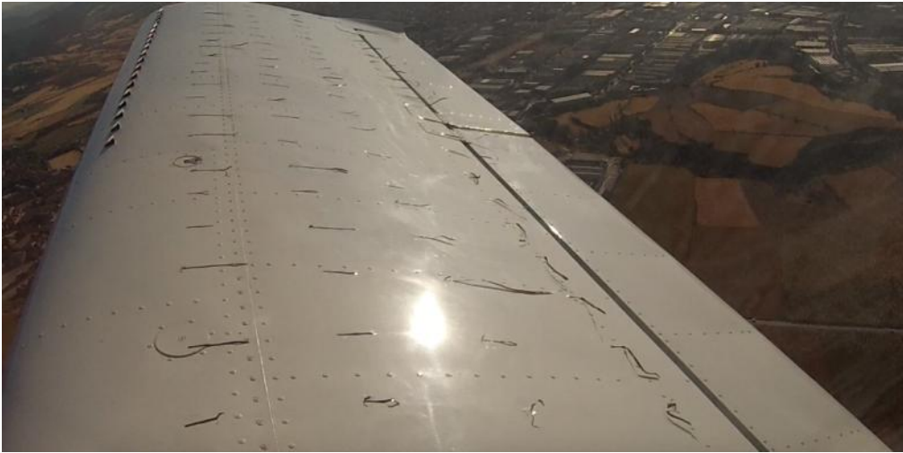
Figure 58: Experimental tests with VG: stall progression
