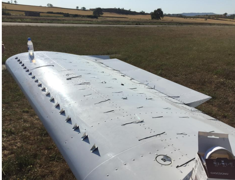
Figure 53: Wing setup of the ultralight used for flight tests
