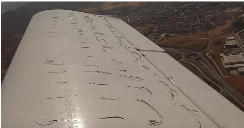
Figure 56: Experimental tests without VG: fully stalled wing
