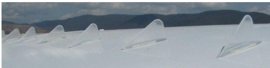
Figure 2 Close-up image of triangle-shaped vortex generators
