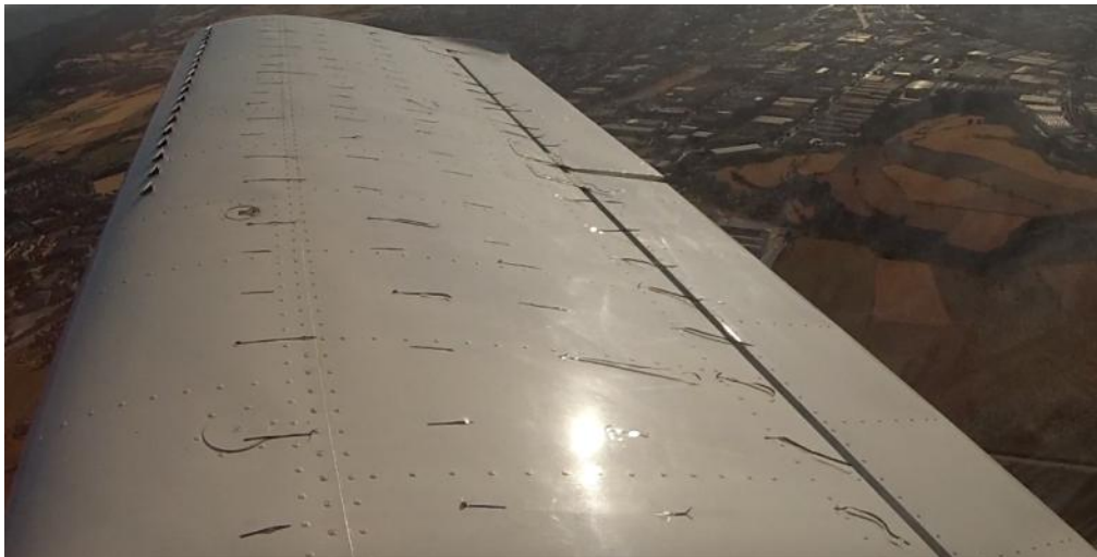
Figure 57: Experimental tests with VG: low speed flying
