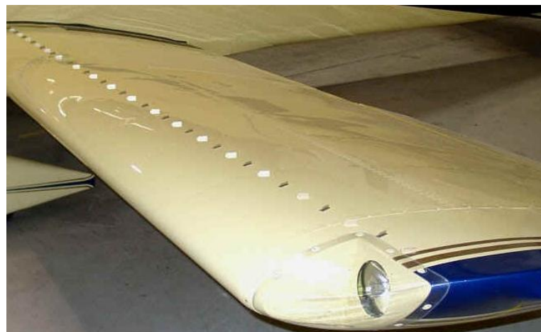
Figure 16: Vortex generators devices mounted along an ultralight wing.
