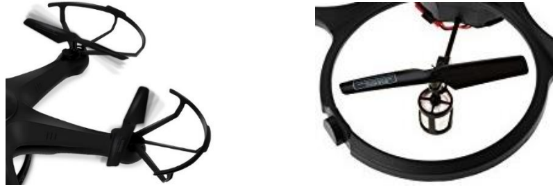
Figure 17 - Examples of fairings in UAVs
