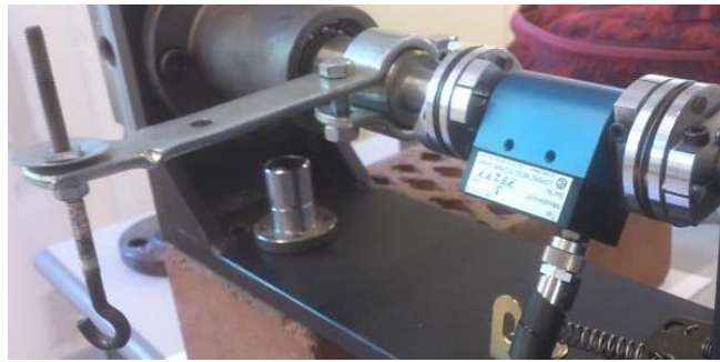
Figure 77 Detailed view of horizontal arm, hook and torque sensor attached to the metal shaft
