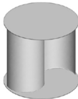
Figure 2 Schematic of a Savonius rotor geometry [1]
