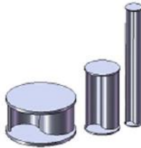
Figure 8 Savonius rotors with different aspect ratios [7]
