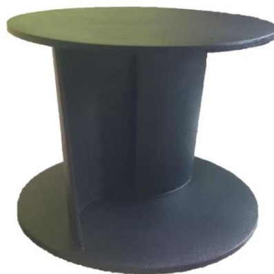
Figure 39 View of the final Savonius rotor after being painted
