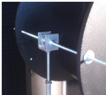
Figure 51 Detailed view of the angular positioning system (APS)
