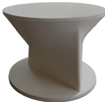
Figure 35 Final rotor printed with the support material
