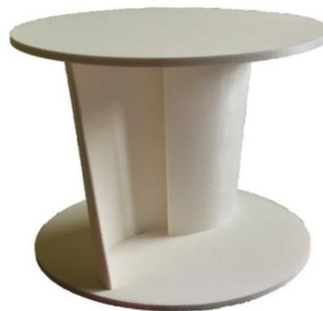
Figure 37 Final rotor printed without the support material
