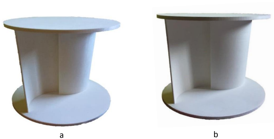
Figure 38 View of the Savonius rotor with (a) the acetone applied on its surface and (b) with the plastics primer applied
