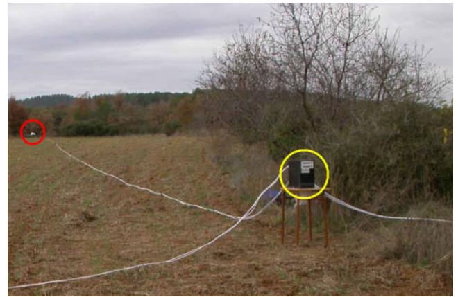
Fig. 3 Test setup overview: Antenna 1 (red circle) and data logger (yellow circle). Cables connecting the antennas and the data logger are 100 m long and are 120° apart.
