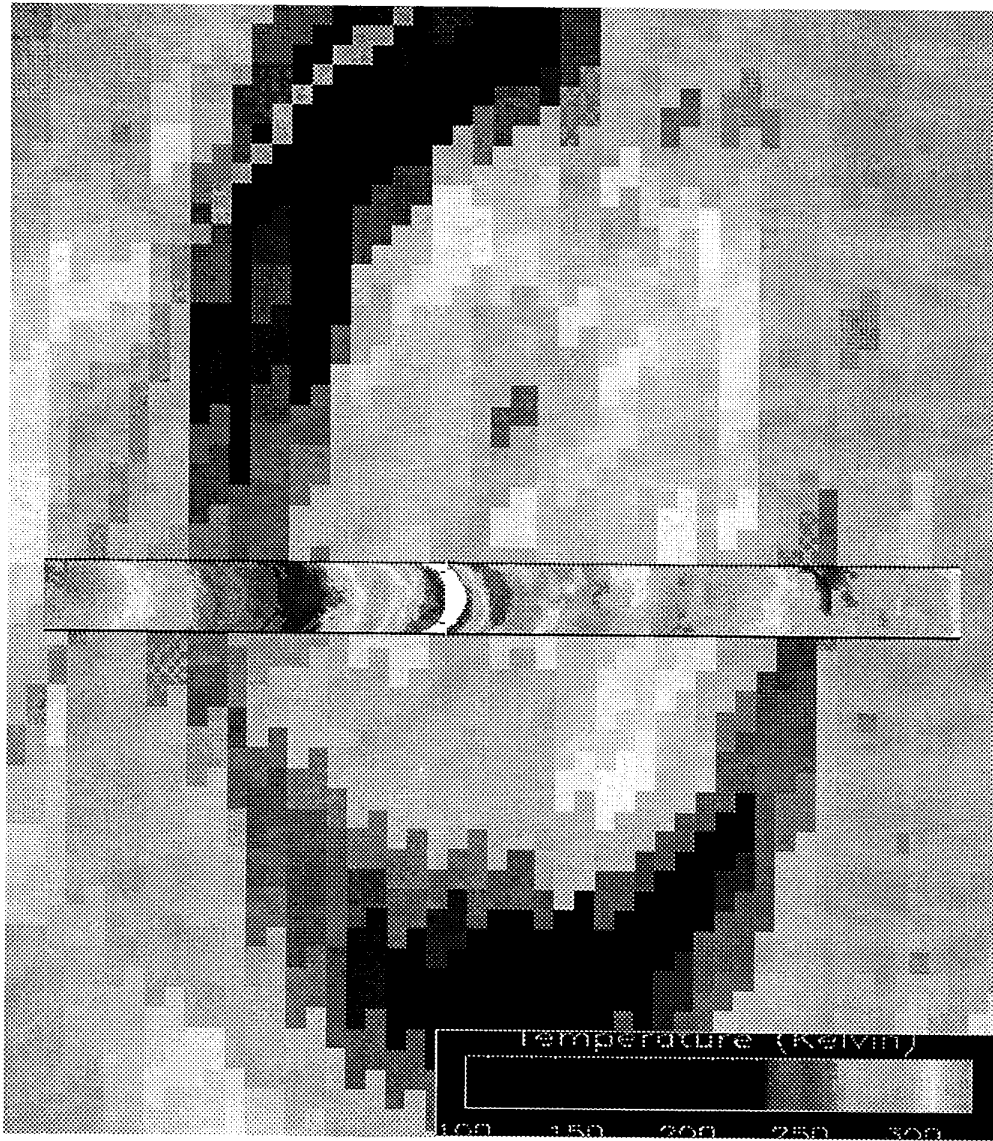
Figure 2. 89 GHz from the PSR pass at 1400-1425 GMT overlaid on the 85 GHz from DMSP F14's SSM/I image from 1358 GMT.
