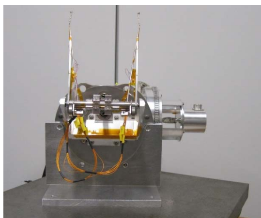
Figure 3.15: Image of the PS scanner; the geometry of the fork can be clearly appreciated.
