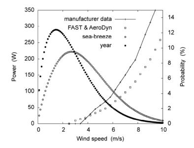
Figure 4. For the HP-600W: manufacturer power curve and power curve obtained from FAST and AeroDyn, together with Weibull distributions for the entire year and the sea breeze period (March 1 to September 30, 10 to 19 LT) as obtained from wind speed data measured in the Llobregat Delta from 1993 to 2010.
