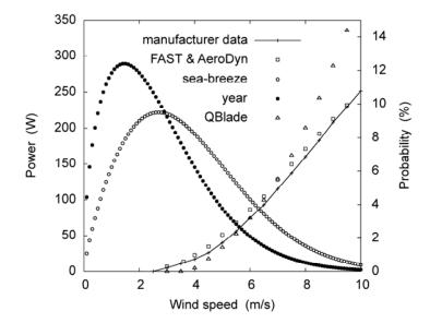
Figure 3. For the IT-PE-100: manufacturer power curve and power curves obtained from FAST and AeroDyn, and from QBlade, together with Weibull distributions for the entire year and the sea breeze period (March 1 to September 30, 10 to 19 LT) as obtained from wind speed data measured in the Llobregat Delta from 1993 to 2010.
