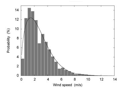
Figure 1. Wind speed distribution and fitted Weibull probability density function for the entire year (January 1 to December 31, 00 to 24 LT) as obtained from wind speed data measured in the Llobregat Delta from 1993 to 2010.
