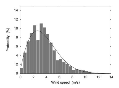
Figure 2. Wind speed distribution and fitted Weibull probability density function for the sea breeze period (March 1 to September 30, 10 to 19 LT) as obtained from wind speed data measured in the Llobregat Delta from 1993 to 2010.
